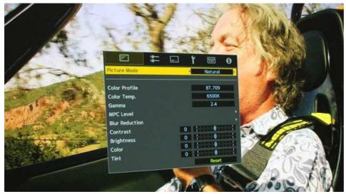
The Z1 automatically recognised an HDR stream of *Luke Cage* (Netflix), playing via a Panasonic DMP-UB900 UHD Blu-ray player, and adopted the appropriate HDR10 profile. When content swaps from HDR to SDR, it then drops back automatically.
